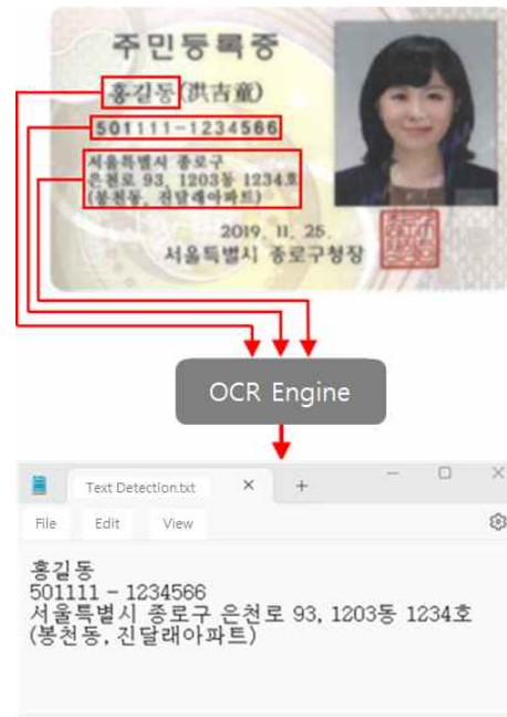
* The figure contains Korean characters to explain the process which converts Korean character of input image into Korean text data using OCR engine as an example.
