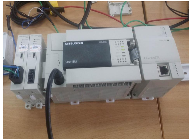
Fig 7. The interface is attached to form a PLC
